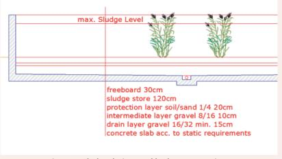
Figure 4: Sludge drying reed bed - cross section
