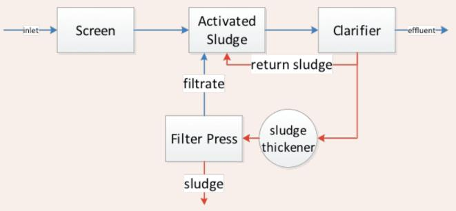
Figure 1: Current flow scheme
