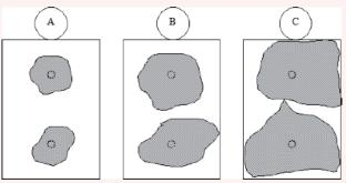
Figure 3: Plan view of surface layer area evolution in a bed of Glandieu during 12 day assay. Circles represent feeding points, from no surface layer at day 0 to (a) day 2; (b) day 4; and (c) day 12. Adapted from Chazarenc and Merlin (2005).
