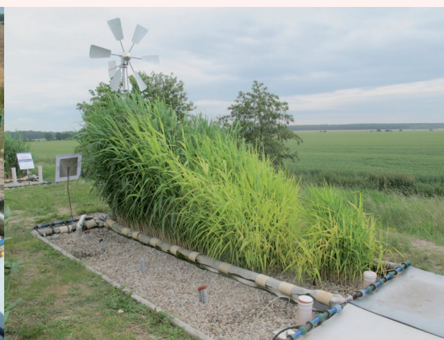
Figure 5b: Langenreichenbach horizontal flow forced aeration reed bed, receiving settled effluent: progressively shorter, yellower reeds further from inlet (13Jun13)
