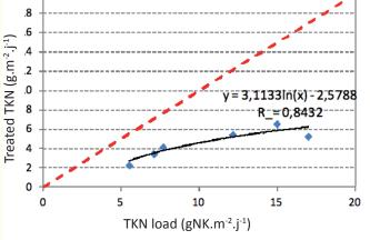
Figure 9: Treated TKN on the first stage for 0.1 < HL < 1.57 m/d.
