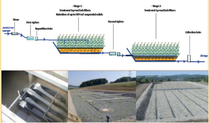
Figure 3: VF CW configuration with siphon
