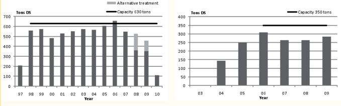
Figure 2: Sludge production and sludge load (left: Helsinge, right: Nordborg)
