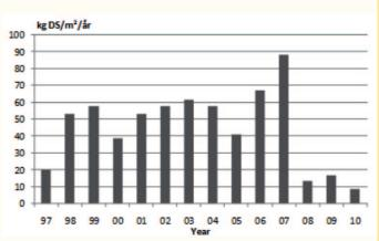
Figure 3 Helsinge Sludge Reed Bed System (basin no.1) Average area loading rate (kg DS/m<sup>2</sup>/year)
