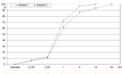
Figure 1: Sieve Analyses Filter Sand at Matany Hospital
