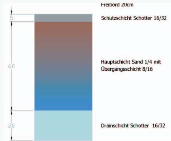
Figure 5: Vertical flow constructed wetland (left) and the layers of the vertical flow bed (right).
