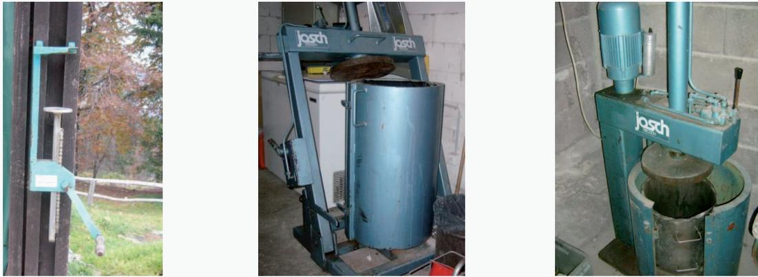
**Figure 3: different kinds of waste presses used in mountain refuges: simple press for cans (left), hand operated waste press (middle), electrically driven press (right) (photos IEVEBS)**
