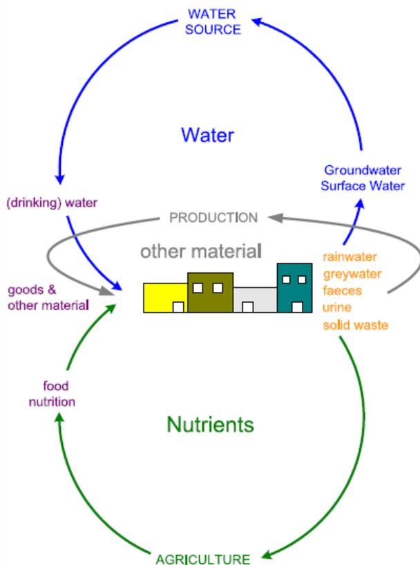
**Figure 2: Resources-oriented or ecological sanitation system (Langergraber and Müllegger, 2005)**
